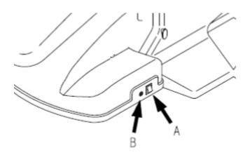
The fuse are placed on the baseplate of the chair, general fuse (B, picture above), can be easyly replaced without open a covers, before to replace the fuse, make sure that main power switch (A picture above) shall be off. More fuse are placed on the Power supply PCB.
