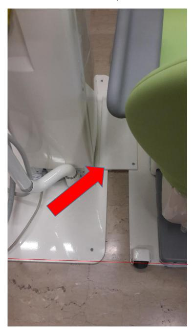
**4.** Lock the chair on the ground using the pedal.
