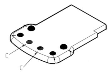
If that button is pressed, the chiar goes automaticly to the rinsing position, by pressing it again after rinsing the chiar goes to the latest position has been in use.
