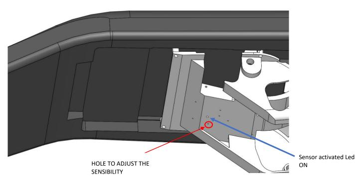
When the sensor is activated while the chair or backrest is driving down, the movement get stop and a sounds beep (bip-bip) inform that the safety backrest chair is activated; a Led (blue colour) (located under the seat) gets on, and stay "ON" up to the safety is activated.
