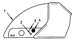
To replace the fuse inside the unit, is needed to remove the cover (1) by removing the screw (3)
