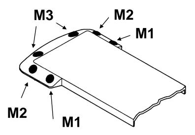
How to call the Pre Set M1, M2 o M3, if the chair position is different to **ZERO POSITION**, Is needed use the following buttons in the following way.
